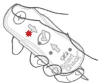
5. When you see the flashing green light, close the inflation valve. The green light indicates that set up is complete.
